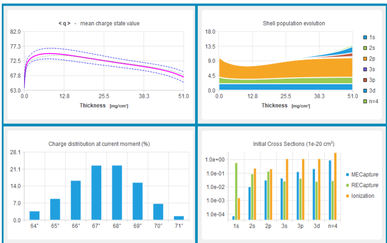
Fig.1. ETACHA4-GUI charge state evolution plots for a ^{207}\text{Pb} projectile at energy 28.9 MeV/u with initial ionic charge 64^+ going through a carbon degrader of thickness 51 mg/cm 2 .
