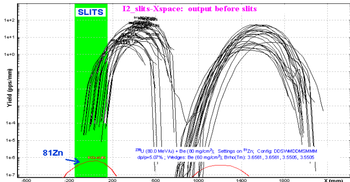
Fig.112. Horizontal spatial distribution plot of fission fragments in the reaction ^{238}\text{U}(80\text{MeV/u})+\text{Be}(80\text{mg/cm}^2) using an achromatic Be-wedge ( 60\text{mg/cm}^2 ) in the intermediate dispersive focal plane (the dispersion is negative).
