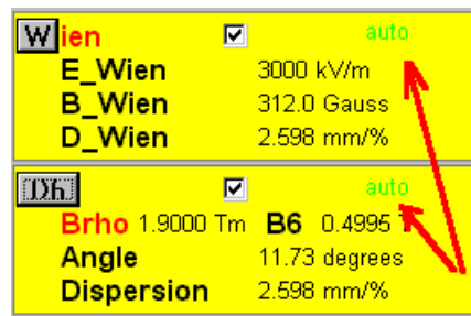
Fig.687. Window of adjustments: installed flags AUTO show, that calculations of parameters of the Wien filter and dipole D6 occurs automatically to changes of the setting fragment and magnetic rigidity of the second dipole.
